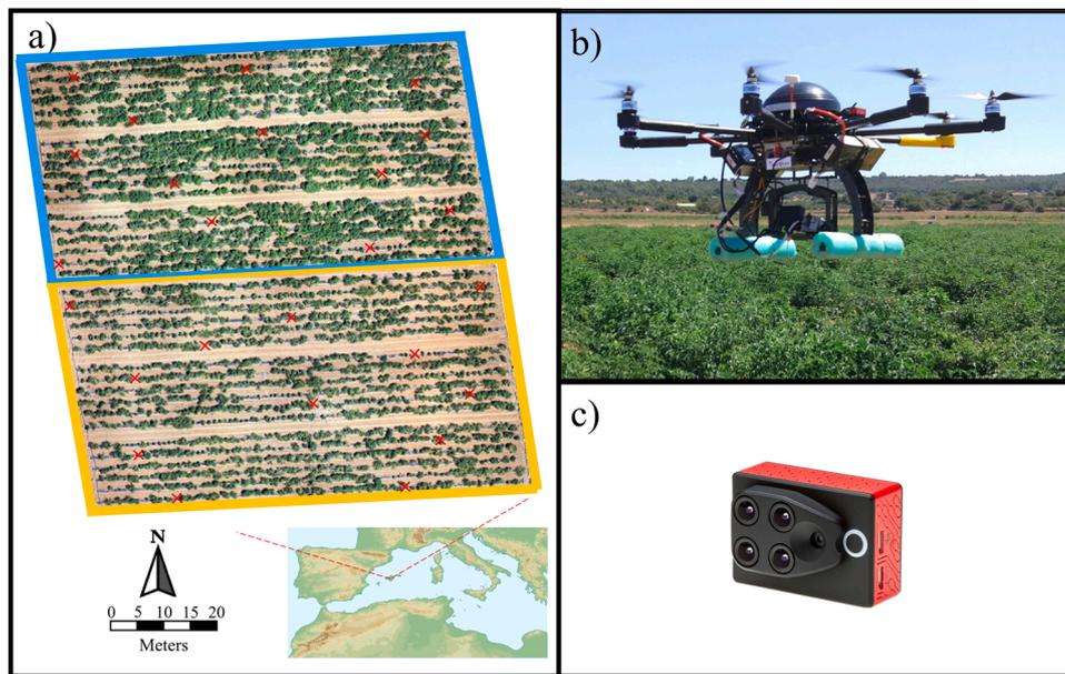
**Fig. 1.** Images of a) the location of the study (blue square delimits the well-watered treatment and yellow square the water deficit treatment; red crosses indicate the location of the ground control points in the field), b) the UAV (FV8, Atyges, Malaga, Spain) and c) the camera used to obtain the multispectral images (Parrot Sequoia sensor, Parrot SA, Paris, France).
